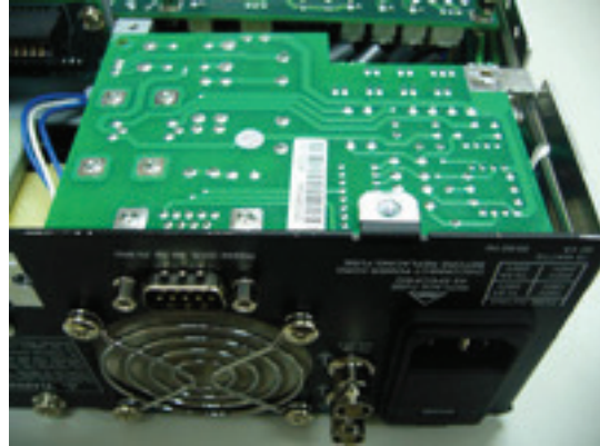
DC Power Supply PCB (FG01P020)
